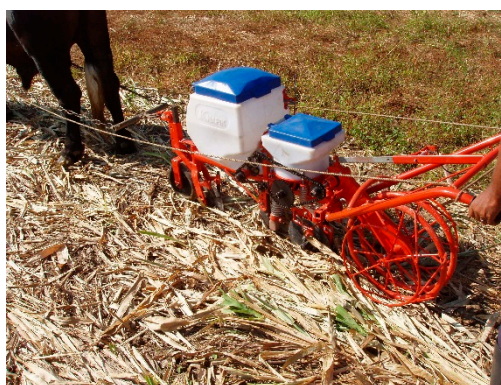
Figure 4. Knapik animal-drawn no-till planter with double offset disc openers to better cut through heavy surface residue (Brian Sims).
