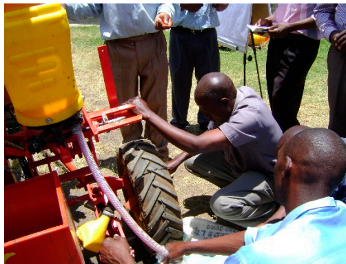
Figure 16. Static calibration of a no-till planter (Brian Sims).
