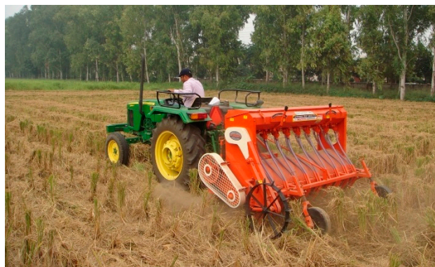
Figure 3. Tractor-mounted Turbo-Happy Seeder with rotating flails to cut residue in front of the chisel-tines and simultaneously clean each side of the tine as the rotor spins, the rotating parts do not touch the soil [15] (Harminder Singh Sidhu).
