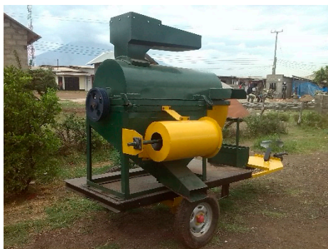
Figure 18. MUST sheller/chopper developed by the Centre for Agricultural Mechanization and Rural technology (CAMARTEC), Tanzania. The machine is trailer mounted and hauled between sites by a 2WT (Wilson Baitani).
