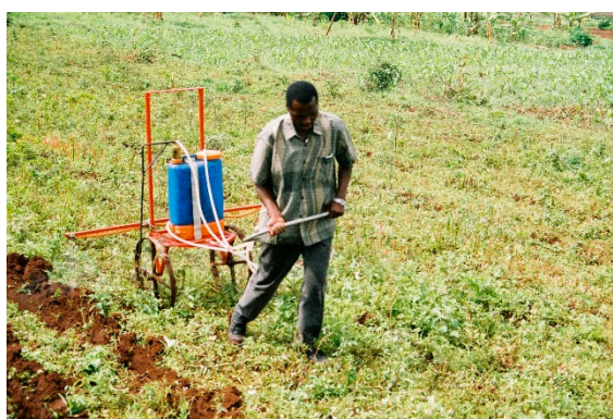
Figure 9. Knapsack sprayers can be modified to become hand-pulled units which not only apply herbicide more uniformly but also keep the operator well clear of the spray (Brian Sims).
