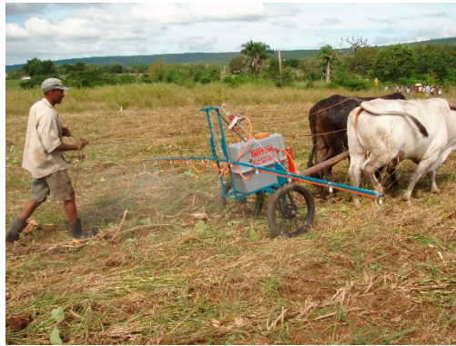
Figure 10. Larger sprayer units with bigger tanks and wider spray booms are available commercially for animal traction (Brian Sims).
