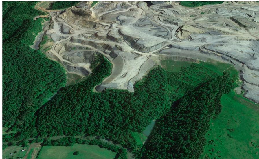
**Figure 2.** Two Valley fills side by side near Chavies, Kentucky [37.373367, 83.351092]. Valley fill is an engineered earthen and rock structure where excess soil and rocks are deposited from surface mining or, in some cases, underground mining. They built in approximately 1995 (right) and 2013 (left). They are 350 m and 300 m deep, respectively. Source: Google Earth.
