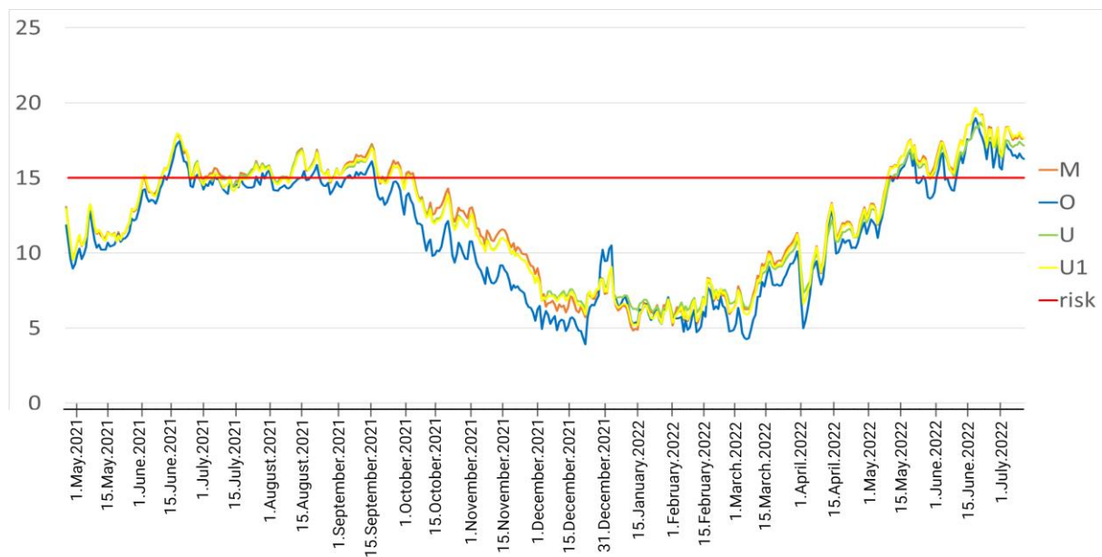
Figure 5. Graphical representation of daily average temperatures throughout the complete study period with data from all temperature loggers. The red line (risk) represents the cutoff value of 15 °C temperature, which is critical for PKD in trout. Daily average temperatures from all loggers were calculated, and each color represents one temperature logger. As visible, during the summer months, the temperatures were above the red line for many consecutive days and weeks. Regarding the loggers, the water in the upstream location was always cooler compared to the other three locations. Abbreviations: Aug—August; Sept—September; Oct—October; Nov—November; Dec—December; Jan—January; Feb—February.
