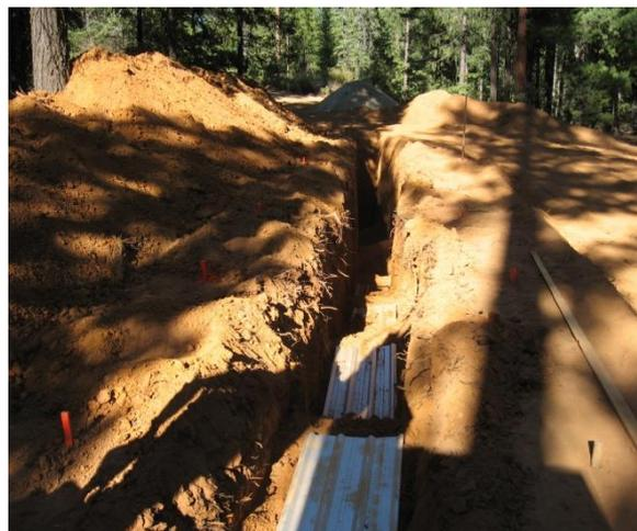
**Figure A1.** Target ground penetrating radar (GPR) imaging objects, tin roofing sheets, were buried at various depths. The experiments provided ground truth GPR data for hardware to software comparison [1,4].
