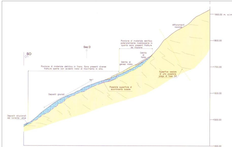
Figure 3 – Geological profile of the Stadelte landslide (from Agency 3, May 2010).
