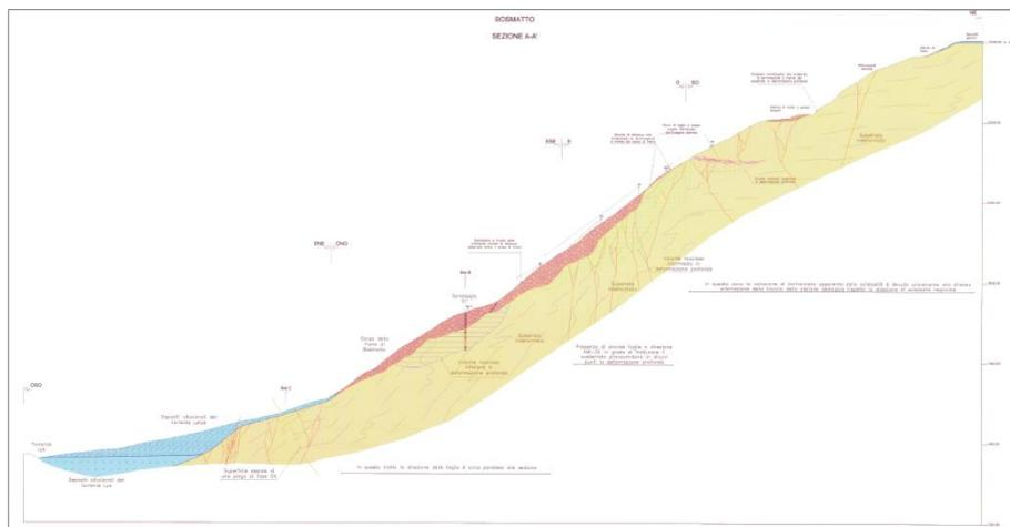
Figure 4 – Geological profile of the Bosmatto landslide (Agency 3, May 2010).
