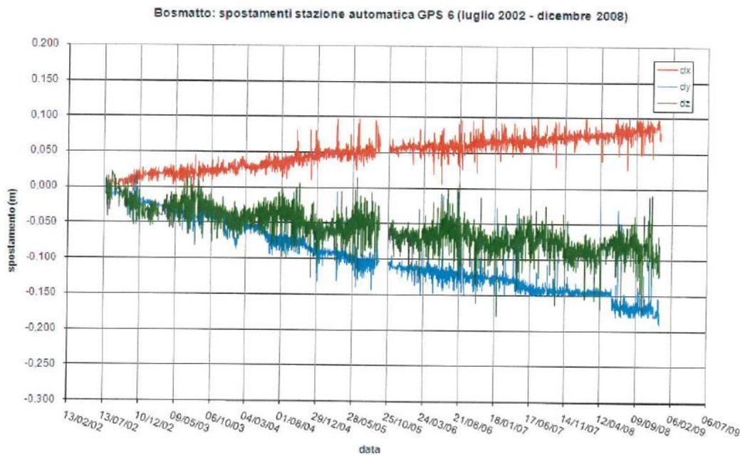
Example of ground deformation time series presentation, relative to an automated GPS (Agency 3, May 2010). The graph reports the three displacement components East, North and altitude from July 2002 to August 2008.
