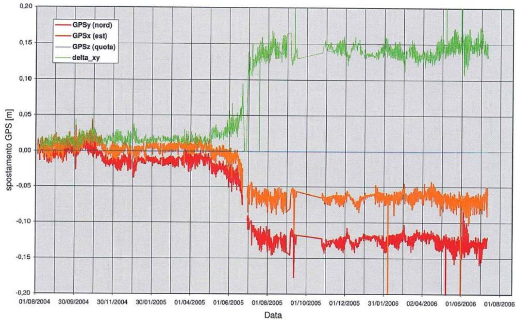
Example of ground deformation time series presentation, relative to an automated GPS (Agency 2, November 2006). The graph report the East, North, planimetric and altimetric time series of the Stadelte GPS from August 2004 to July 2006
