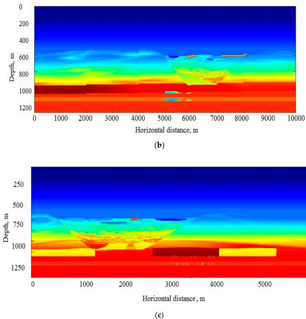
**Figure 4.** 3D heterogeneous multiscale geological model: paleo channel overrides fractured reservoir. (a) Horizontal cross-section at the depth 800 m, (b,c) two orthogonal vertical cross-sections through the middle of the model.
