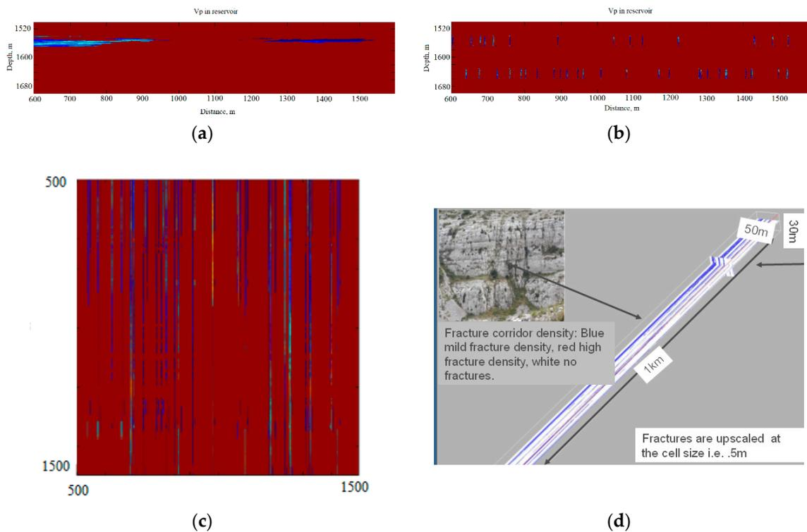
**Figure 5.** Sketch of the reservoir. (a–c)—side and top views. (d) Upscaling of the fractures to fracture corridors.
