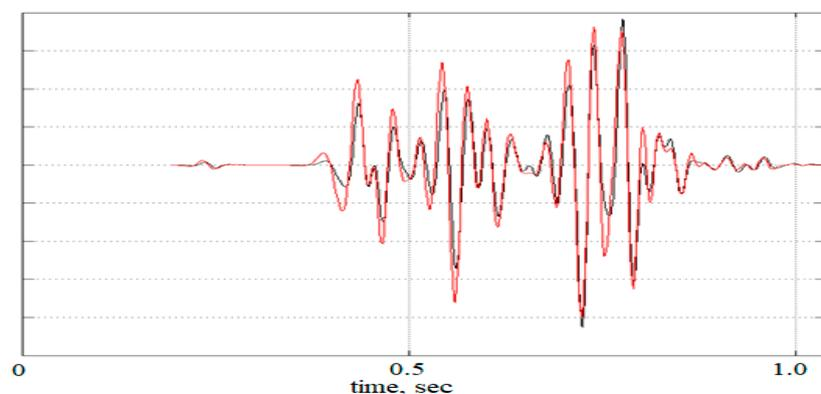
**Figure 8.** Comparison of a zero offset trace, computed by full finite difference simulation (black) and exploding reflectors approach (red).
