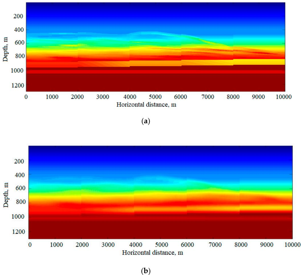
**Figure 6.** The vertical cross-section of the paleo-channel model. (a) No smoothing (b) After smoothing.
