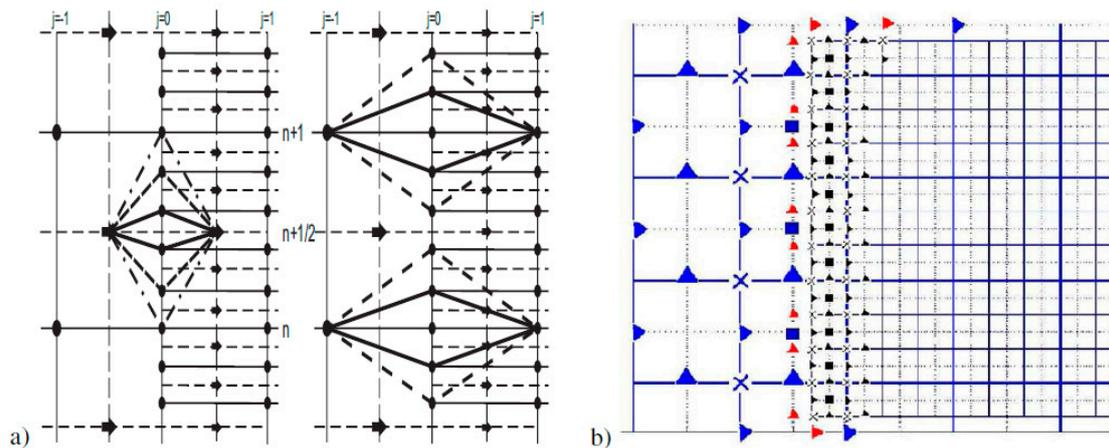
**Figure 2.** The mutual disposition of fine and coarse grids. (a) In time, (b) In space.
