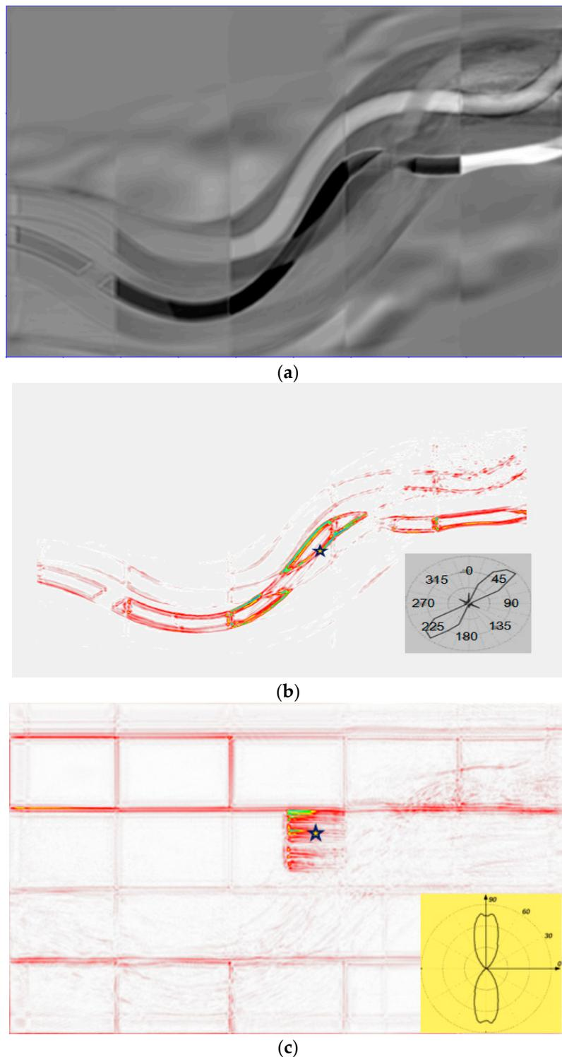
**Figure 9.** (a) Poststack time migration image at  $t = 0.5$  s. (b) Poststack time domain diffraction image at  $t = 0.5$  s. (c) Poststack time domain diffraction image at  $t = 0.84$  s.
