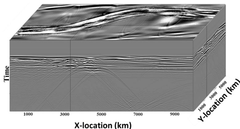
**Figure 10.** Zero-offset cube computed by the adaptive FD scheme for the model shown in Figure 5.
