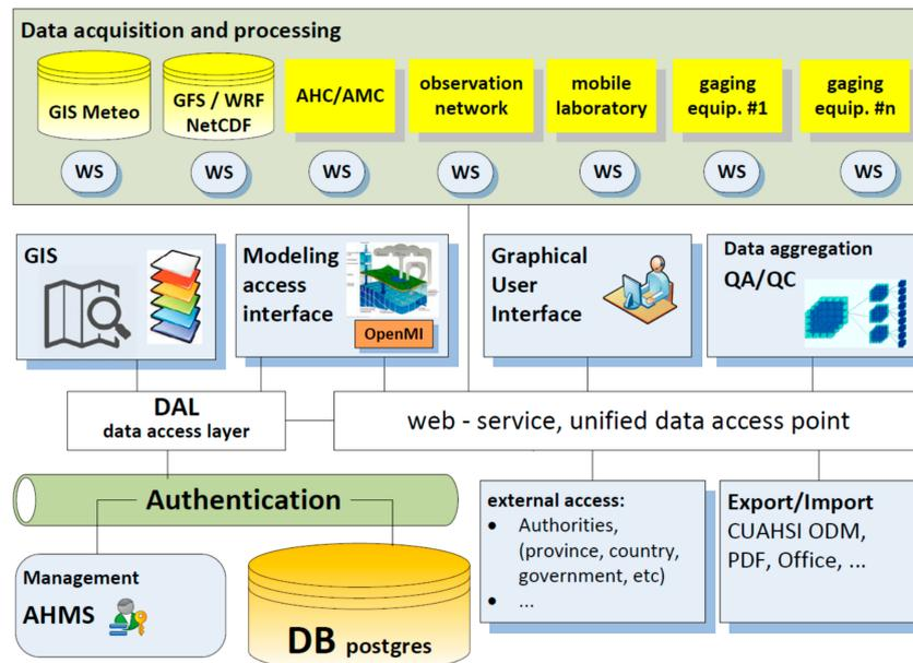
**Figure 2.** Flow-chart of local AHMS server (AHC/AMC—automatic hydrological/meteorological complex, WS—windows service; DAL—data access library, QA/QC—quality assurance/quality control).
