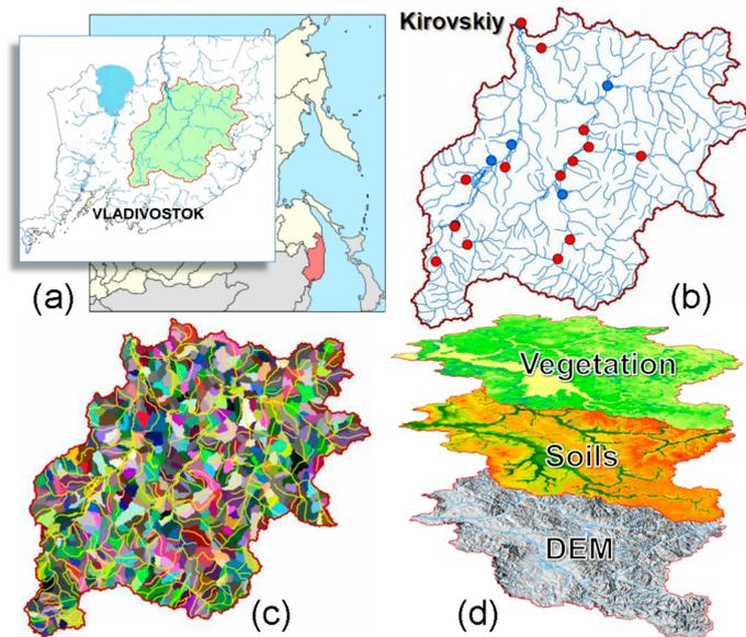
**Figure 4.** Upper Ussuri River Basin position (a) and information set; (b) observational network (red circles weather stations, blue circles hydrological gages); (c) ECOMAG model unit schematization and (d) DEM, soil and vegetation map coverages.
