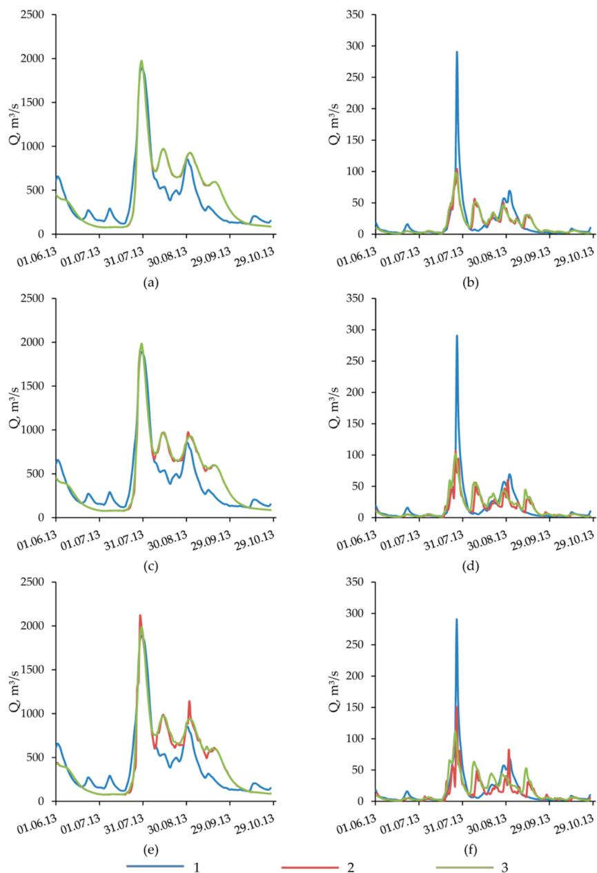
**Figure 5.** Examples of observed (1) and forecasted (2—with precipitation gradations, 3—with WRF data) runoff hydrographs of 2013 year in gaging stations Ussuri-Kirovskiy (a,c,e) and Krylovka- Krylovka (b,d,f) with lead time at 1, 2 and 3 days, accordingly.
