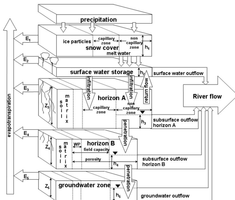
**Figure 1.** Schematic representation of water pathways in ECOMAG elementary watershed.
