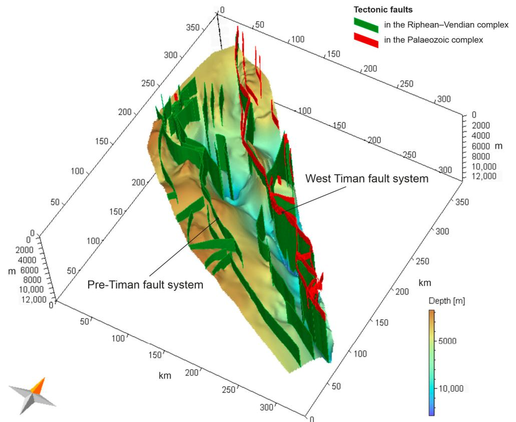
**Figure 2.** Three-dimensional structural model of the Vychegda Trough on the basement surface with a system of tectonic faults.
