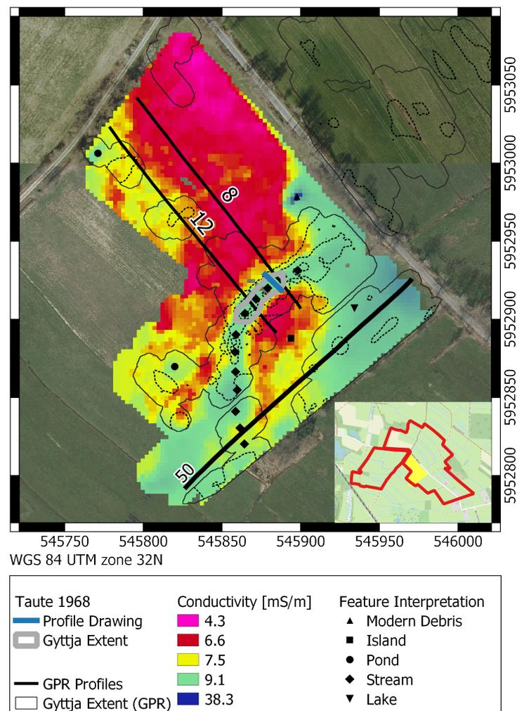
**Figure 12.** Joint interpretation of Electromagnetic Induction and Ground-Penetrating Radar data. The electrical conductivity of the first coil pair (i.e., averaged over the first ~1.2 m of the subsoil) is colour coded. The extent of the gytja deposits as derived from GPR interpretation is delineated in black. Depth contours of the gytja base at 0.5 m intervals are provided as dashed black lines.
