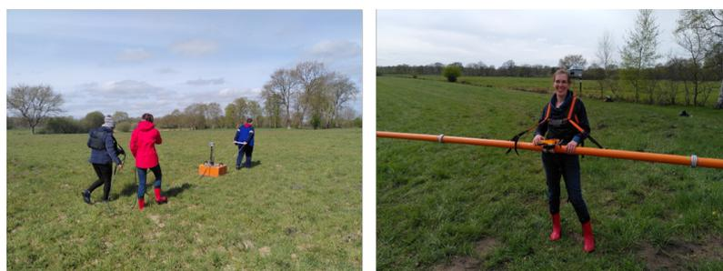
**Figure 3.** Impressions from the geophysical fieldwork in Lieth Moor. (Left): GPR measurements are performed by dragging the 200 MHz antenna across the ground. (Right): EMI measurements were conducted with the device carried at waist height, approximately 1 m above the ground. Photos: Stine Detjens.
