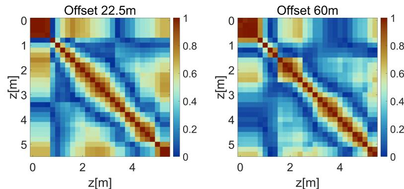
**Figure 10.** Covariance correlation coefficients of 1D EMI inversions at 22.5 m and 60 m offset within GPR profile 12 (cf. dashed lines in Figure 9). For this test, the number of best models used to calculate the covariances was increased to 200. Reddish colours indicate a high trade-off between modelled conductivity values at the respective depth locations.
