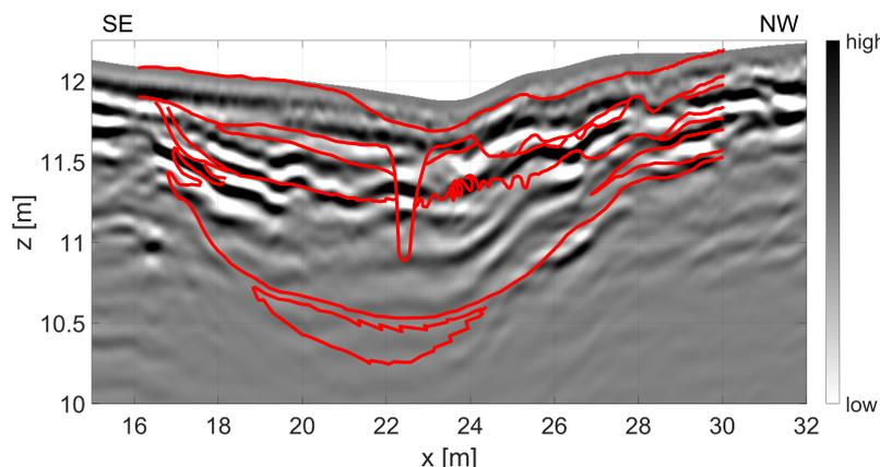
**Figure 13.** Comparison of GPR signal and Taute’s section. A detail from GPR profile 8 is overlain with the sedimentary profile drawing from ([66], p. 74). The drawing is parallel projected onto the nearest GPR profile. For information on the location, see Figure 12. The distance between GPR profile and excavation is ca. 3 to 5 m.
