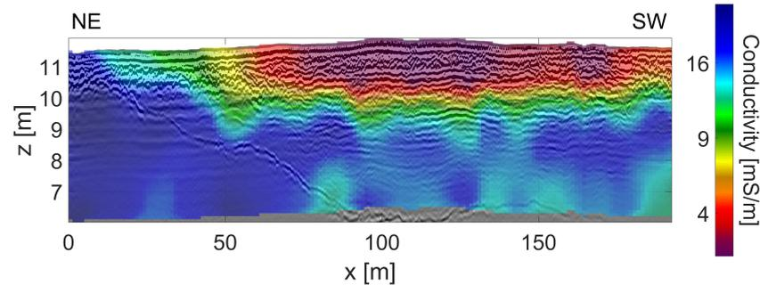
**Figure 11.** Electric conductivity depth section overlain on GPR reflection profile 50. The electric conductivity section was obtained through an inversion computation from the EMI data. Again, the colourmap is root scaled for better visibility of the major features within the dataset (denoted conductivity values are corrected and in mS/m).
