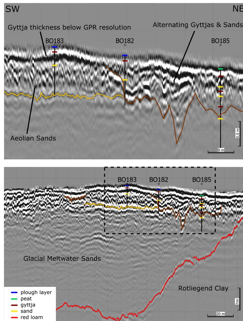
**Figure 6.** GPR profile 50 and adjacent cores. Top: enlarged detail of the uppermost 2 metres. The red line shows the top of the ‘red loam’, which emerges extremely close to the surface towards the northeast. The brown line denotes the base of the limnic gyttja and sand facies. Additionally, within this specific subarea, an extra reflector beneath the aeolian sand facies is discernible and is delineated by the yellow line.
