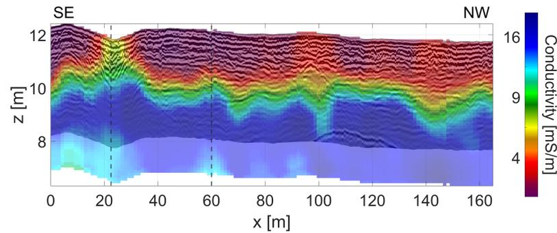
**Figure 9.** Electric conductivity depth section overlain on GPR reflection profile 12. The electric conductivity section was obtained through an inversion computation from the EMI data. For better visibility of the major features within the dataset, the colourmap is root scaled (denoted conductivity values are corrected and in mS/m). Dashed lines refer to the locations of the covariance correlation coefficient tests shown in Figure 10.
