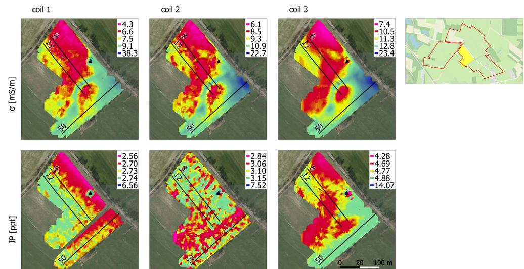
**Figure 8.** EMI data after processing. This figure illustrates the electrical conductivity ( $\sigma$ ; top) and inphase (IP; bottom) data obtained from the three coil pairs, presented from left to right. Black lines indicate GPR profiles 8, 12 and 50. An upward triangle denotes the location of extreme inphase and increased conductivity values, which we assign to modern construction debris. In the overview map of the study area, the displayed subarea is drawn in yellow.
