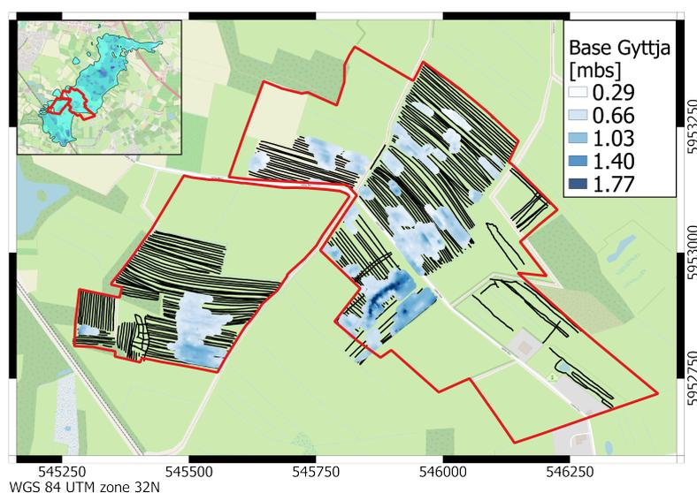
**Figure 7.** Depth of the gyttja base in metres below ground surface as derived from GPR profile interpretation.
