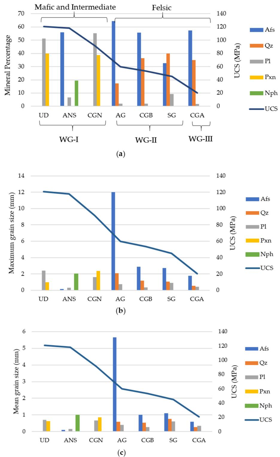
**Figure 6.** Relationship between the petrographic characteristics, weathering grade, and strength. (a) Effect of mineral composition and weathering grades on the strengths of mafic, intermediate, and felsic rocks. (b) Effects of maximum grain sizes of minerals and weathering grades on the strengths of mafic, intermediate, and felsic rocks. (c) Effects of mean grain sizes of minerals and weathering grades on the strengths of mafic, intermediate, and felsic rocks.
