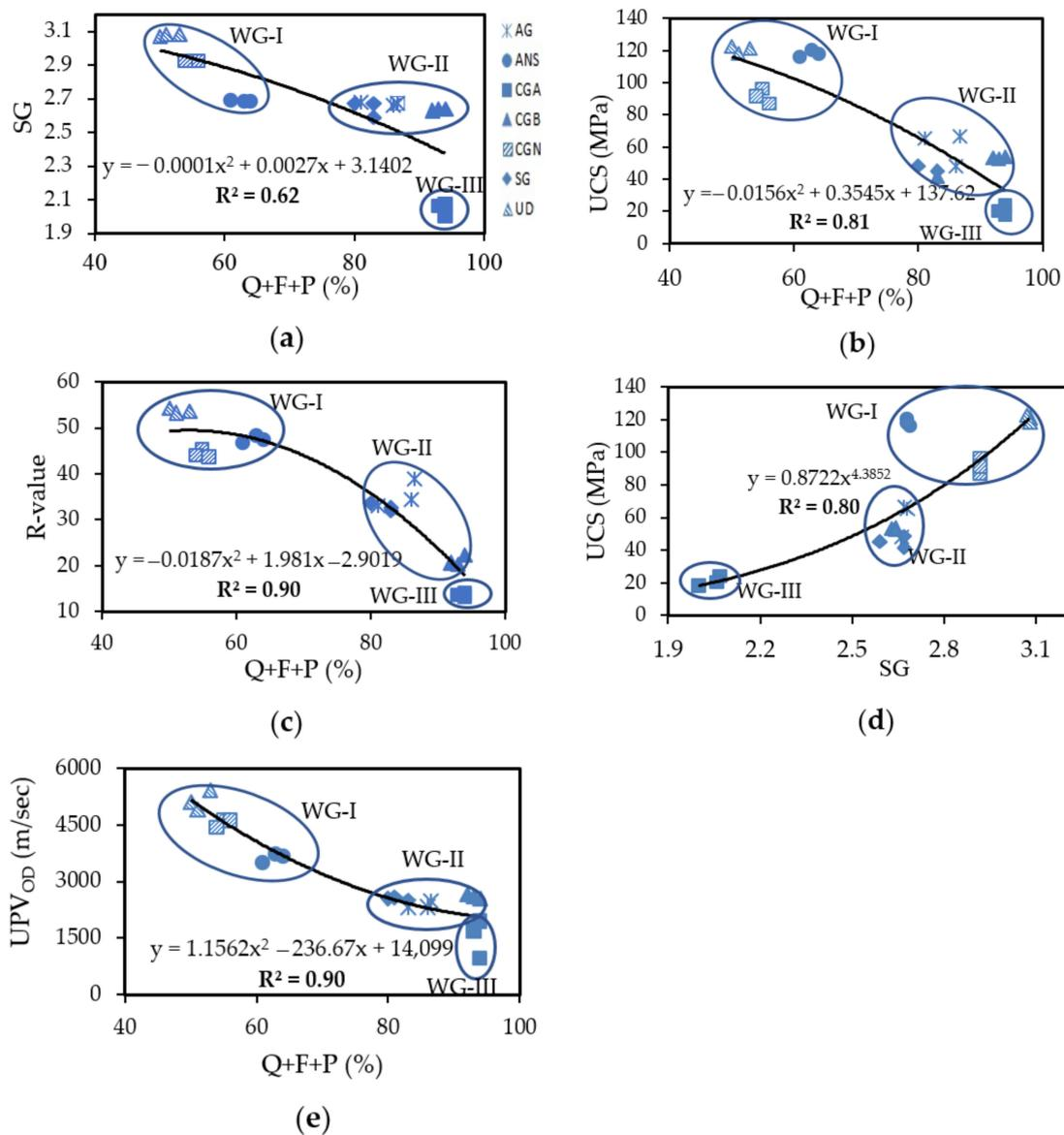
**Figure 4.** Correlation plots of (a) cumulative percentage of quartz, feldspar, and plagioclase (Q + F + P) vs. specific gravity (SG) (polynomial), (b) Q + F + P vs. unconfined compressive strength (UCS) (polynomial), (c) UCS vs. SG, (d) Q + F + P vs. R-value (polynomial), (e) Q + F + P vs. ultrasonic pulse velocity oven-dry (UPV OD) (polynomial). Symbols given in (a) are the same for all figures.
