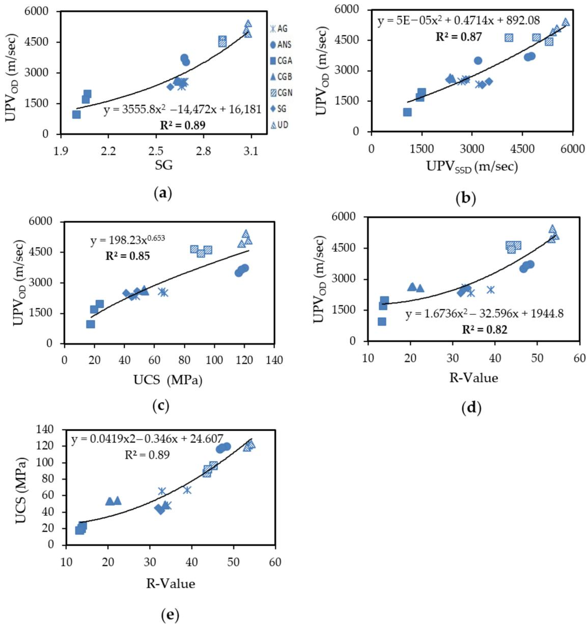
**Figure 5.** Correlation plots of (a) ultrasonic pulse velocity oven-dry (UPV<sub>OD</sub>) vs. specific gravity (SG) (polynomial), (b) UPV<sub>OD</sub> vs. UPV<sub>SSD</sub> (polynomial), (c) UPV<sub>OD</sub> vs. UCS (power) (d) UPV<sub>OD</sub> vs. R-Value (polynomial), (e) UPV<sub>OD</sub> vs. R-Value (polynomial). Symbols given in (a) are the same for all figures.
