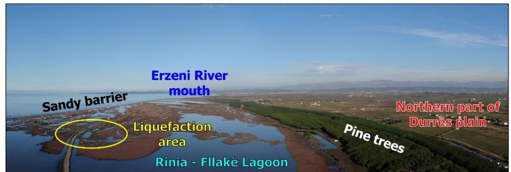
**Figure 9.** Drone view of the Rinia–Fllakë Lagoon. The sites with the detected liquefaction phenomena are also noted along with the main geomorphological features of the lagoon.
