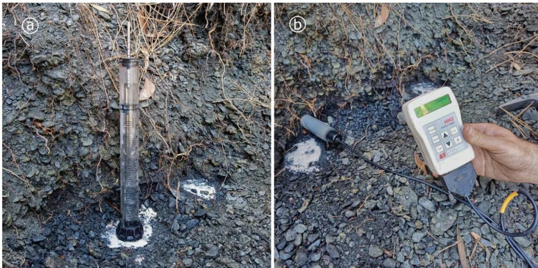
**Figure 4.** Field measurements of soil unsaturated hydraulic conductivity (a) and volumetric water content (b).
