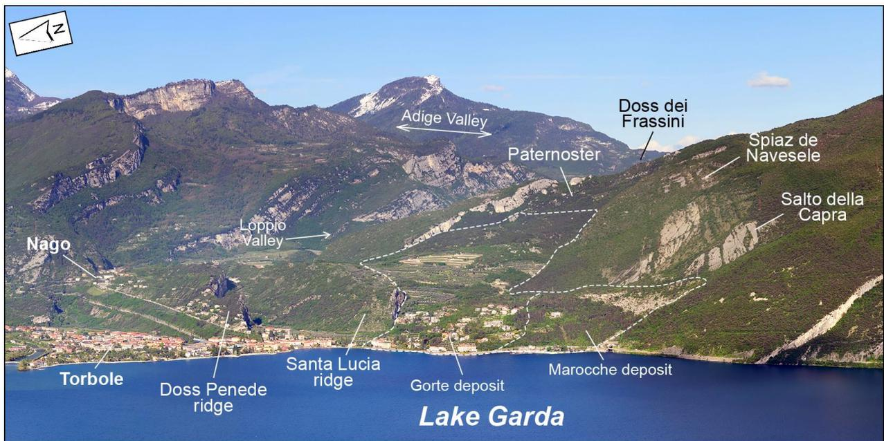
**Figure 3.** Overview of the landslides of Gorte (on the left) and Marocche (on the right). The latter is due to the visible sliding planes of the Spiaz de Navesele and Salto della Capra. Mouth of the Sarca River seen on the far left of the image. Photo taken from the western side of Lake Garda (photo courtesy of Dr. Matteo Visintainer).
