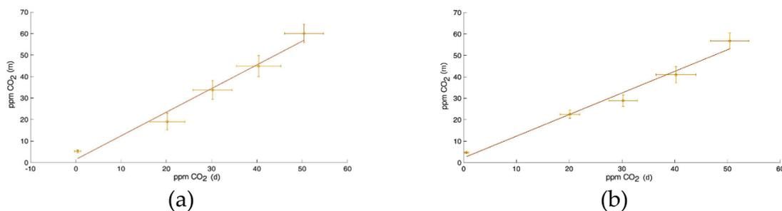
**Figure 4.** The best-line fits of the two tests: the first, (a) reports the increasing concentration test, while the second, (b), the decreasing concentration test. In both figures, the x axis (ppm  $\text{CO}_2$  (d)) reports the  $\text{CO}_2$  concentrations driven into the flux chamber unit, while the y axis (ppm  $\text{CO}_2$  (m)) reports the  $\text{CO}_2$  concentrations measured.
