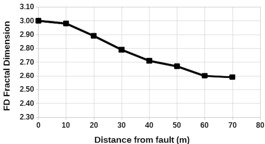
**Figure 7.** Fractal dimension values from the fault (at distance 0) to the different distances.
