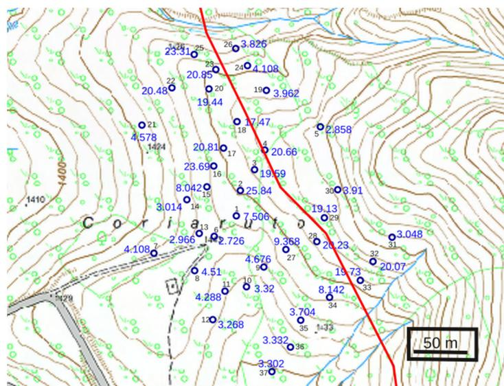
Figure 3. The map of the full set of measurements (flux values in ppm cm<sup>-2</sup> s<sup>-1</sup>), with the fault position [43,44] shown with a red line. The x axis represents the latitude from 42°33'23.436" N to 42°33'38.286" N, while the y axis represents the longitude from 13°22'58.962" E to 13°23'17.3832" E.
