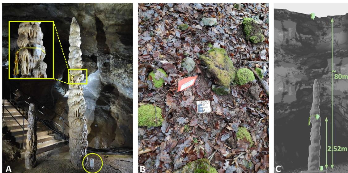
**Figure 3.** Three-component seismic sensors placed for the study of the natural frequency of the Minaret. (a) The two sensors in the cave: with a yellow ratchet strap on the Minaret and placed on the ground next to the stalagmite. (b) The sensor at the surface, in the soil at the vertical of the Minaret stalagmite. (c) Sketch of the relative position of the three sensors (not to scale in the vertical direction).
