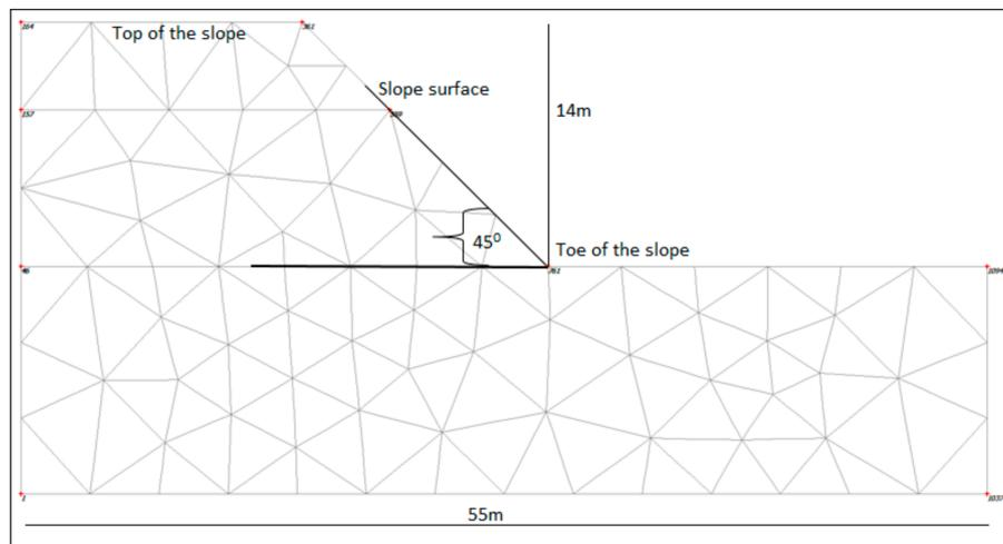
**Figure 5.** Schematic sketch of geometry of the slope, dimensions, discretization and boundary conditions.
