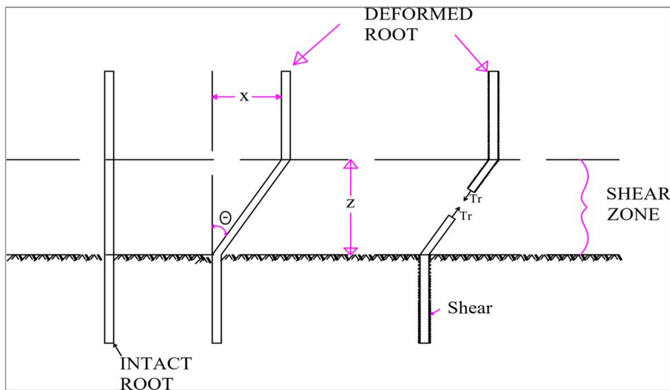
Figure 4. Interface friction between soil and root.
