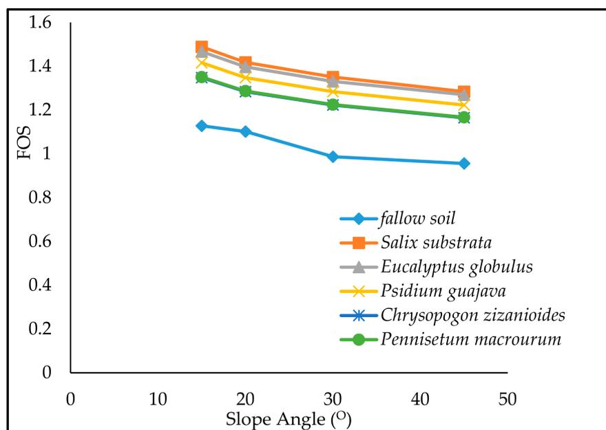
**Figure 12.** Values of the factor of safety for various plant species at different slope angle.
