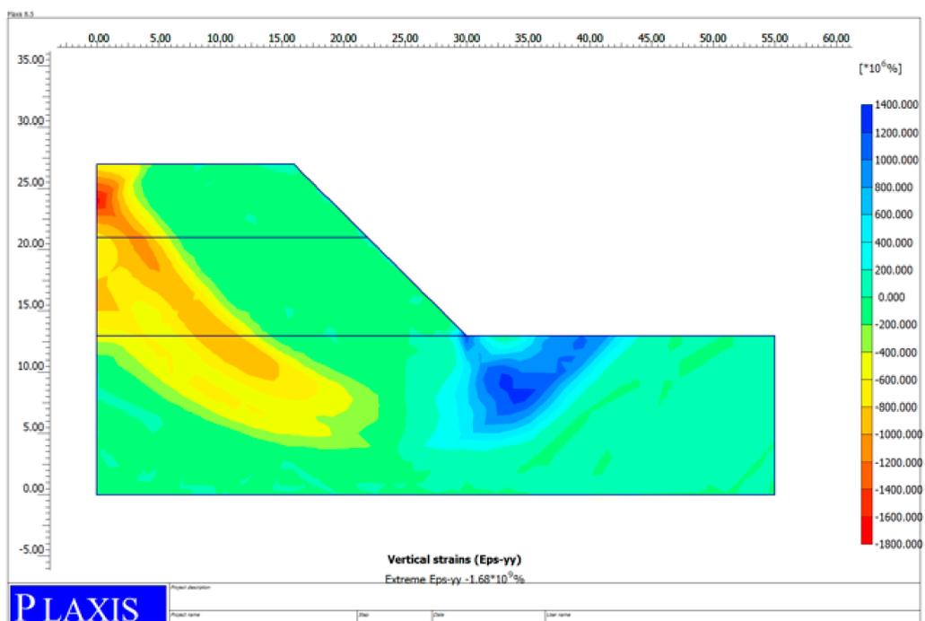
Figure 8. Strain displacement distribution of numerical analysis for non-vegetated slope (*Salix subserata*).
