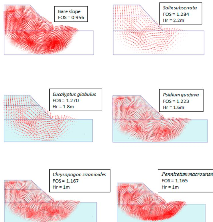
**Figure 6.** Factor of safety for all plant species, in the case of vegetation on entire slope surface.
