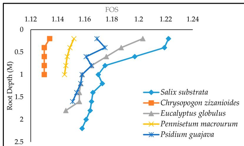
**Figure 9.** The factor of safety vs root depth for all plant species.
