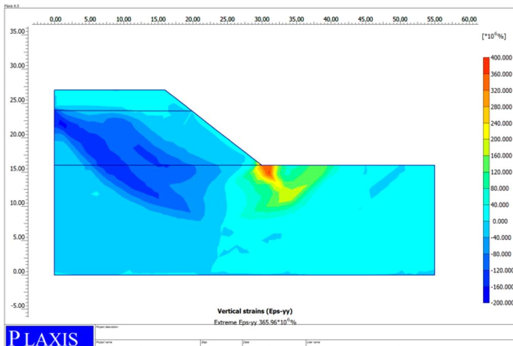
Figure 7. Strain displacement distribution of numerical analysis for non-vegetated slope.
