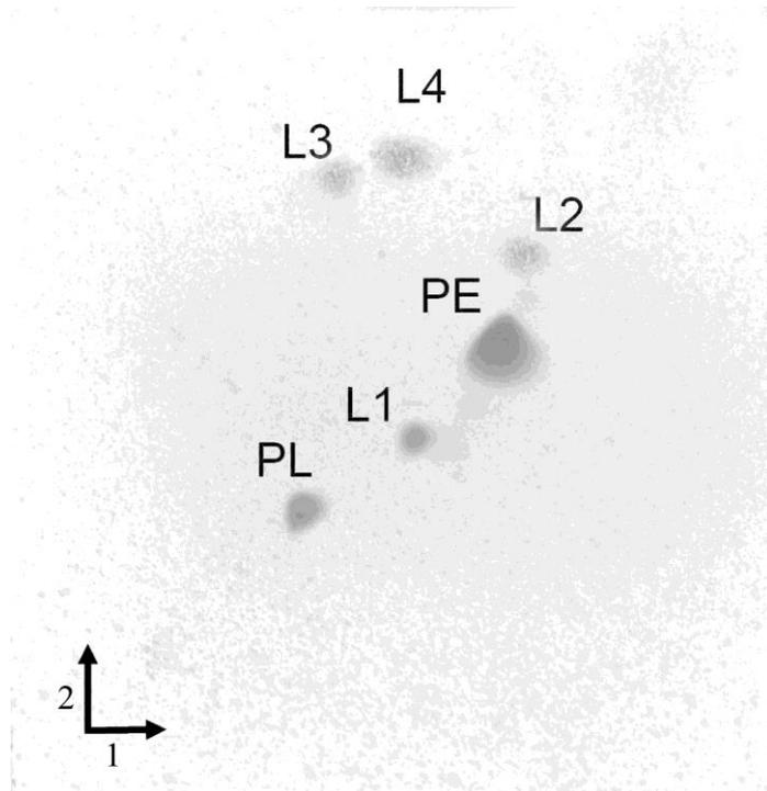
**Figure S1:** Polar lipids of strain GBPx2<sup>T</sup> after two-dimensional TLC and detection with molybdophosphoric acid and heating at 200 °C for 10 min. PE, phosphatidylethanolamine; PL, unidentified phospholipid; L1–L4, unidentified lipids.
