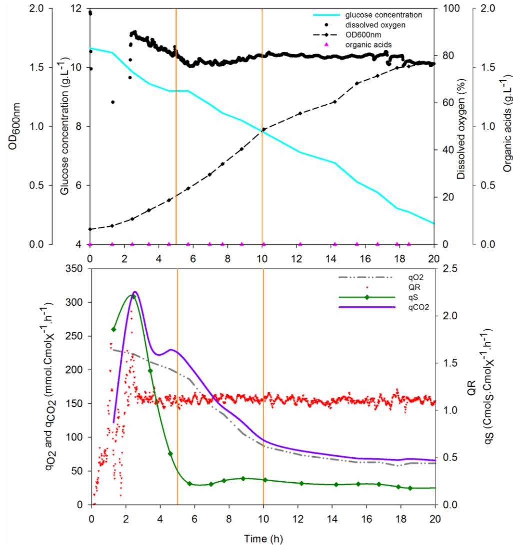
**Figure 3.** Time course evolution of the optical density OD<sub>600 nm</sub>, the glucose concentration, the dissolved oxygen value, the acidic by-products concentration, the respiratory quotient (QR) and the specific oxygen uptake, carbon dioxide production and glucose uptake rates during batch culture of *Deinococcus geothermalis* DSM-11302 (vertical bars represent the three phases of growth).
