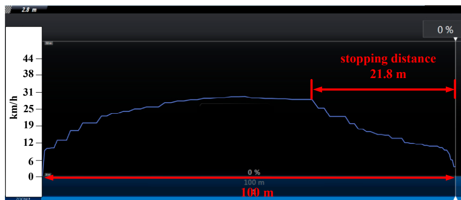
Figure 13. HIL test result of rider of 60 kg, flat road with kinetic brake.
