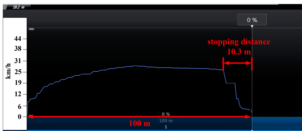
Figure 15. HIL test result of rider of 60 kg, flat road with active regenerative brake.
