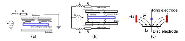
**Figure 2.** Electric levitation micro-actuators based on the passive levitation: (**a**) single-stator design; (**b**) dual-stator design; (**c**) levitation of a charged particle in a hyperbolic oscillating electric field *E* (U is the applied electric potential).
