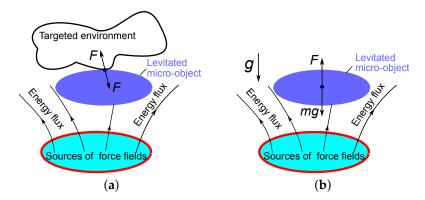
**Figure 1.** Concepts of levitating micro-actuators (*F* is the generated force by the actuator; *m* is the mass of the levitated micro-object; *g* is the gravity acceleration): (**a**) the levitating micro-actuator acting on the environment; (**b**) the levitating micro-actuator acting without targeted environment.
