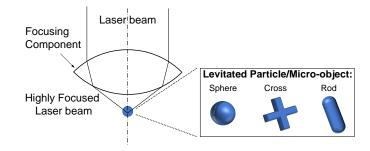
**Figure 6.** Schematic of a highly focused laser beam to create an optical trap and levitate particles or micro-objects. Particles or micro-objects of arbitrary shape (sphere, cross and rod) can be trapped in an optical trap.
