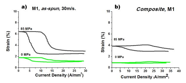
Figure 7. Curves of current density *versus* strain for the: (a) NiTi ribbon, (b) smart composite material.
