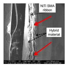
**Figure 4.** Transversal SEM view of the composite material at the union between the magnetic hybrid material and the NiTi ribbon. Red arrows show where adhesion is not fully completed.
