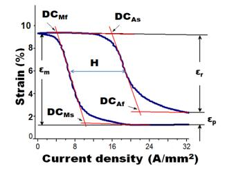
**Figure 6.** Martensitic transformation.  $\varepsilon_r$ : SATWME or strain recovery;  $\varepsilon_p$ : plastic deformation strain; DC<sub>Ms</sub>: start martensite transformation as a function of current density; DC<sub>Mf</sub>: finish martensite transformation as a function of current density; DC<sub>As</sub>: start austenite transformation as a function of current density; DC<sub>Af</sub>: finish austenite transformation as a function of current density; H: hysteresis.
