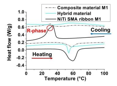
**Figure 5.** Comparison of DSC curves between the magnetic hybrid material, the NiTi ribbon and the composite material M1.
