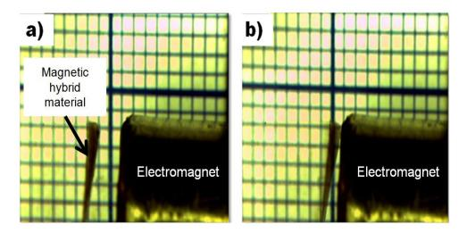
**Figure 9.** Displacement of the composite material when an external magnetic field is applied (top-view). (a) Initial position. (b) Final position.
