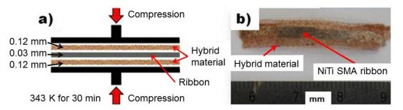
**Figure 3.** (a) Schema of the joining process of the magnetic hybrid film and the SMA ribbon (lateral view). (b) Smart composite material.
