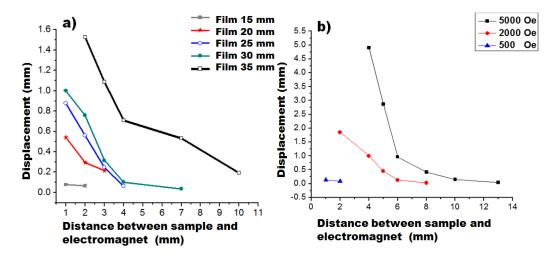
Figure 10. Maximal displacement curves of the samples *versus* the initial separating distance between these and the electromagnet for the: (a) magnetic hybrid film, (b) smart composite material.
