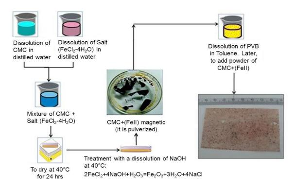
Figure 2. Process to obtain the (Fe<sub>2</sub>O<sub>3</sub>-CMC)/PVB magnetic hybrid polymer.
