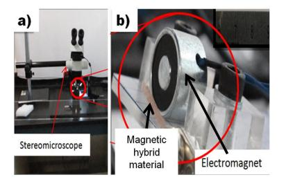
**Figure 8.** Experimental setup for the magnetic experimentations. (a) General view including the stereomicroscope Leica M80. (b) Zoom over the electromagnet and the magnetic hybrid material in a cantilever configuration.
