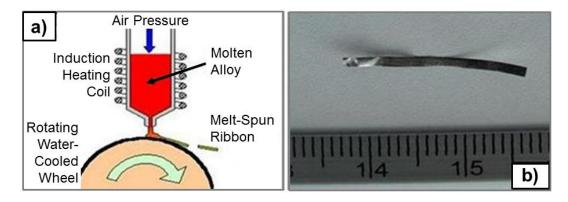
Figure 1. Melt-spinning process. (a) Schema. (b) Resulting NiTi ribbon (measures in mm).
