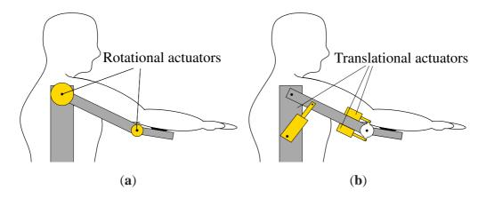
**Figure 3.** Schematic examples of external positioned actuation configuration for (**a**) placed on the stationary part and (**b**) cable suspended.
