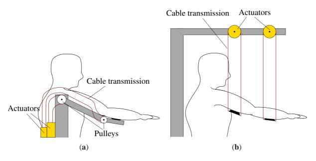
Furthermore, the ROM of all three actuator configurations are comparable except for the cable suspension configuration [55]. Cable suspension can achieve a large ROM with less DOF compared to the other actuation configurations. However, a complete structure covering the user is necessary to achieve this ROM as can be seen in Figure 3b. Designs of cable suspended arm supports are proposed to achieve an optimal ROM [56–58].
