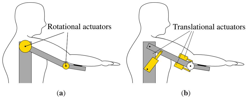
**Figure 3.** Schematic examples of external positioned actuation configuration for (a) placed on the stationary part and (b) cable suspended.
