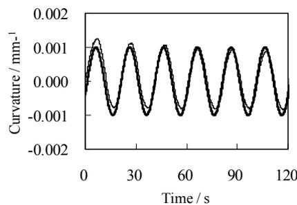
Figure 10a,b again show the bending curvature of a Nafion IPMC specimen under feedforward control along with the imposed current per unit surface area over time, respectively.
