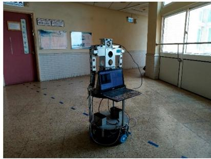
**Figure 24.** After the SURF matching, the robot turns to the target direction and moves forward.
