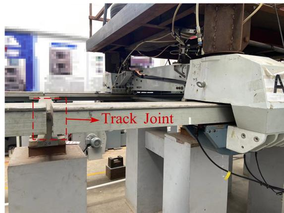
Figure 16. The position of the track joint.
