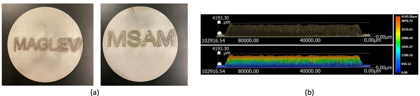
**Figure 5.** (a) Deposition of features on both sides of the levitated geometry. (b) Resulting deposited features from the analysis in Section 5.1
