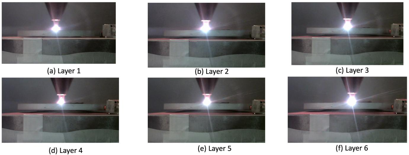
Figure 3. Visual representation of layer-by-layer deposition on the levitated geometry
