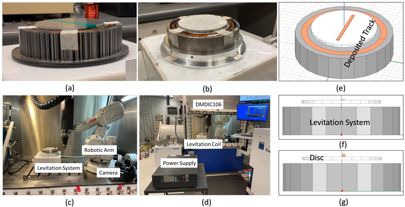
**Figure 1.** (a) Laminated core magnetic levitation system. (b) Solid core magnetic levitation system. (c) Experimental apparatus for magnetic levitation experiment within DMDIC106. (d) Experimental apparatus within the DMDIC106 machine. (e) Simulation model for ANSYS Maxwell—*isometric view*. (f) Simulation model with only one layer—*front view*. (g) Simulation model with 5 layers—*front view*
