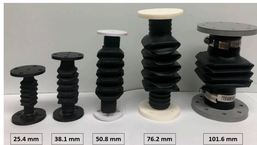
Figure 3. A variety of accordion pattern OSPAs fabricated from different diameter heat-shrink tubes.
