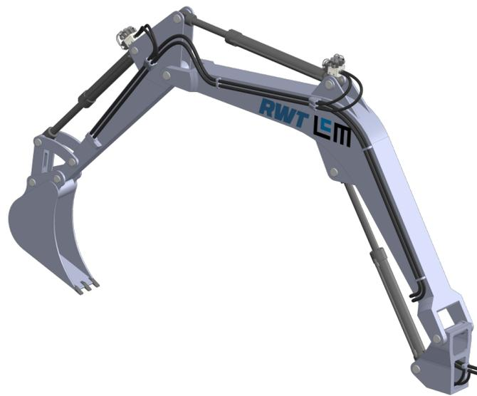
**Figure 11.** Design study of an excavator arm fully equipped with CPS valves.
