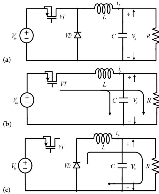
**Figure 1.** Circuit diagram of buck converter. (a) An average case. (b) A switch ON case. (c) A switch OFF case.
