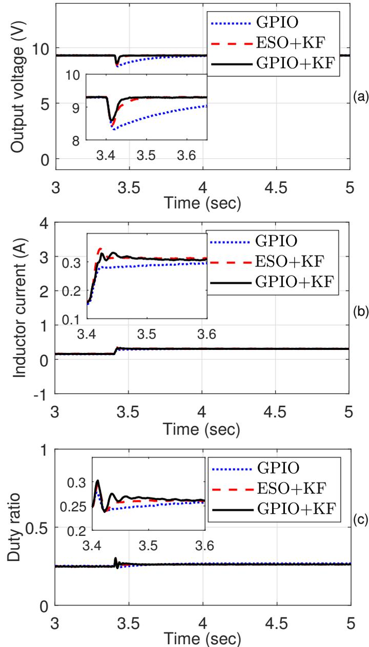
**Figure 4.** Waveform curves when disturbance is form of step. (a) Output voltage. (b) Inductor current. (c) Duty ratio.
