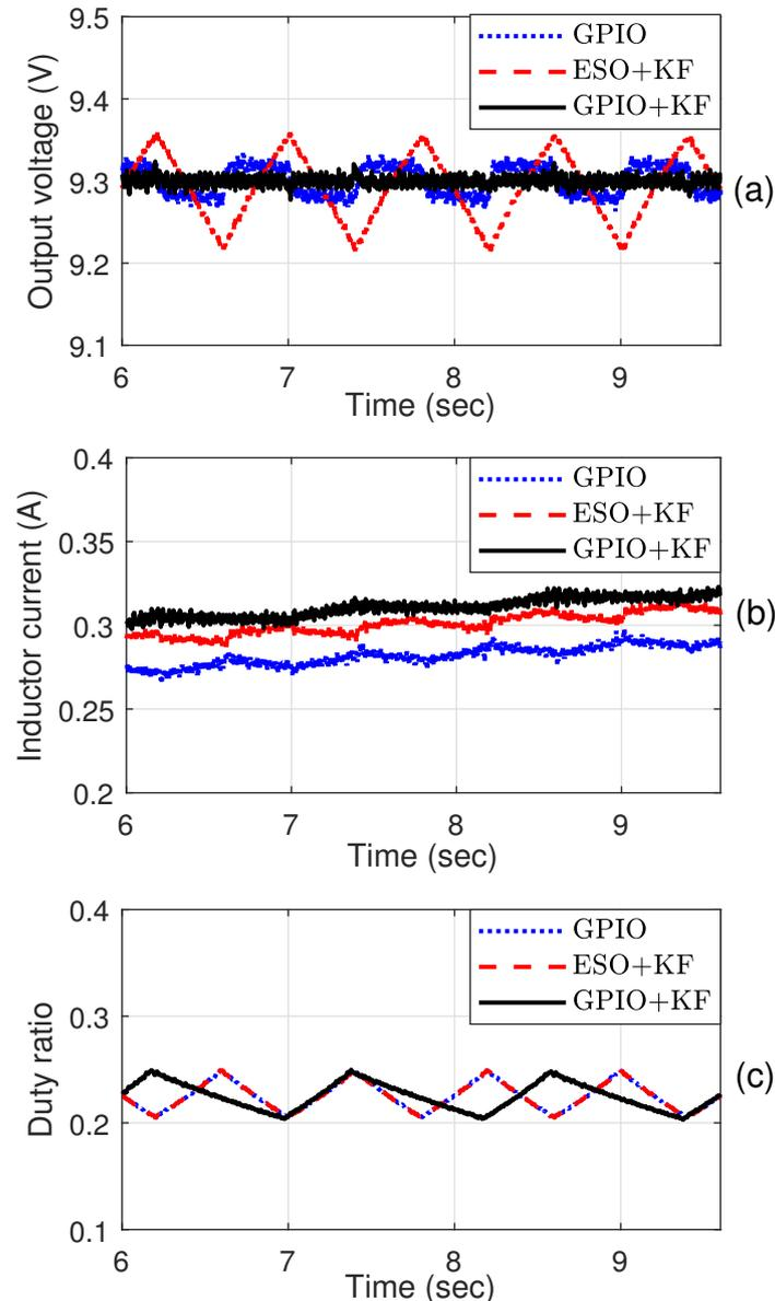
**Figure 5.** Waveform curves when disturbance is polynomial form of time series. (a) Output voltage. (b) Inductor current. (c) Duty ratio.
