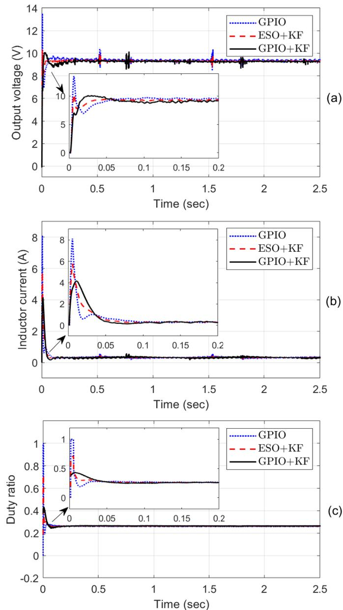
**Figure 3.** Waveform curves when the system is just started. (a) Output voltage. (b) Inductor current. (c) Duty ratio.
