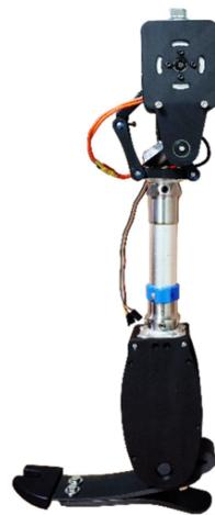
**Figure 7.** Robotic knee prosthesis design assembly.
