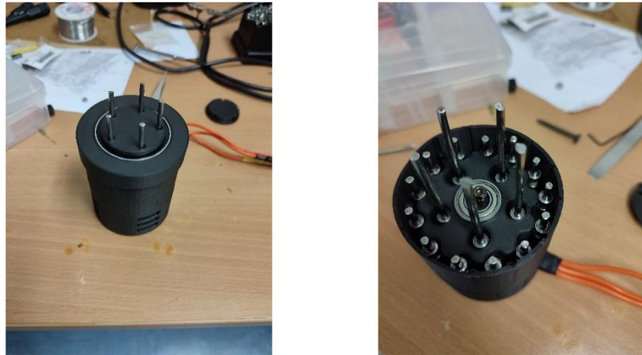
**Figure 3.** Initial assembly of the cycloidal gear drive for testing and load evaluation.
