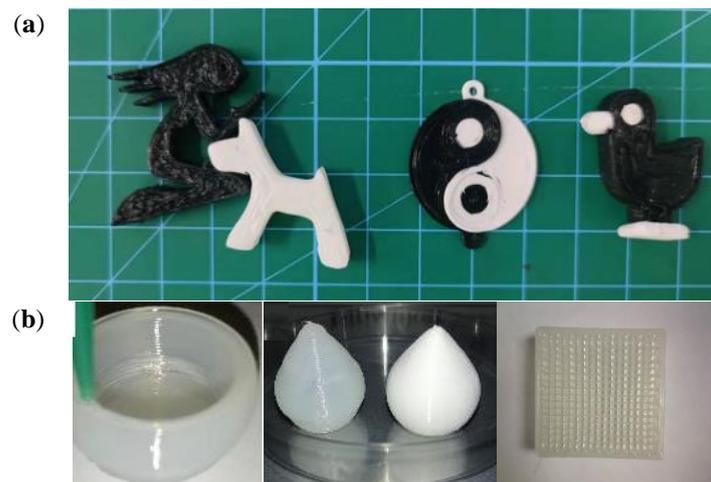
**Figure 7.** (a) Complex 2D structures printed with exemplary silicones; (b) complex 3D structures printed with exemplary silicones.
