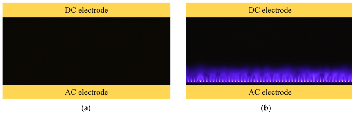
Figure 11. Discharge photographs in the case where a voltage of 10 kV pp at 4 kHz was applied to the AC electrode, and the DC electrode was grounded, in the (a) CD-PA and (b) TED-PA.
