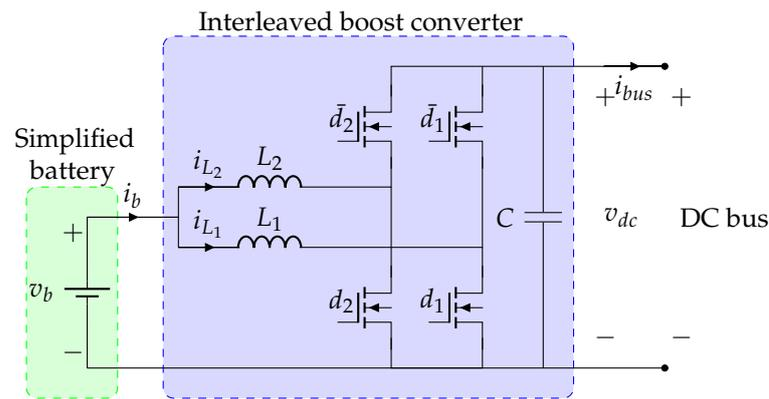
**Figure 2.** Electrical connection of an interleaved boost converter.
