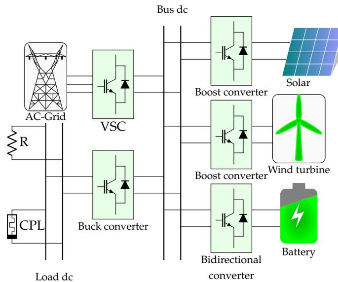
**Figure 1.** A typical DC microgrid with various sources and loads.
