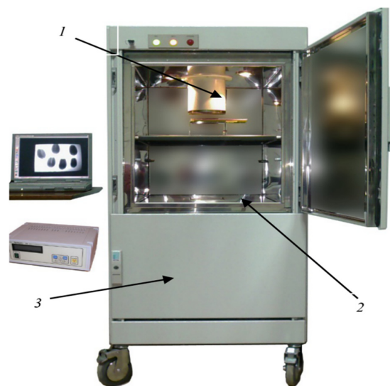
Figure 1. Family PRDU: 1. X-ray source; 2. digital image receiver; and 3. specialized camera for X-ray work.
