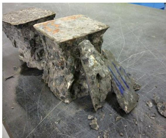
Figure 3. Concrete failure shape after seven days for all specimens.
