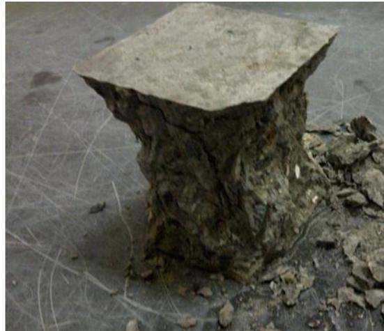
**Figure 4.** Concrete failure shape after 56 days for all specimens.
