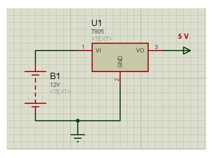
Figure 5. Schematic diagram of the 5 V regulated voltage.
