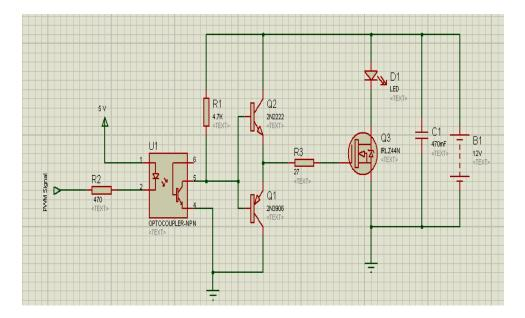
Figure 9. Schematic diagram of LED driving circuit by PWM.
