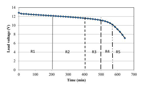
Figure 11. Battery discharge curve regions.
