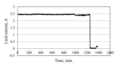
Figure 18. Load current without the smart controller.
