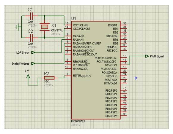
Figure 8. Microcontroller unit circuit with input/output.
