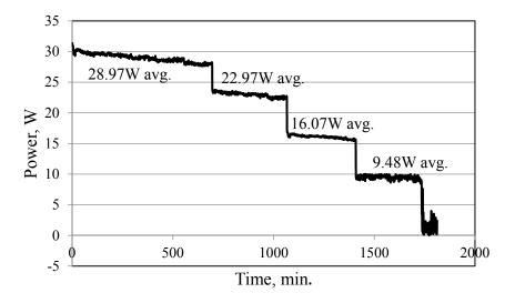
Figure 15. Power of the load during system operation with the smart controller.
