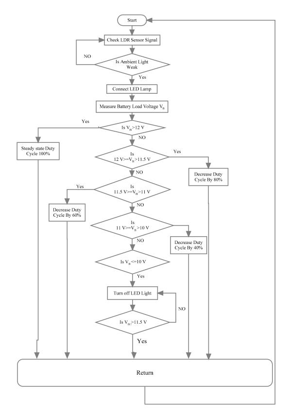
Figure 10. Flowchart of the discharge controller algorithm.
