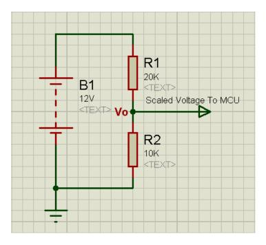
Figure 6. Schematic diagram of a voltage scaling circuit.
