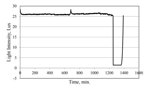
**Figure 20.** Variation of light intensity at the floor directly under the LED and 6 m away without using the smart controller.
