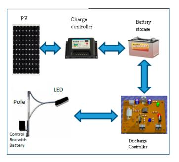
Figure 1. Typical photovoltaic (PV) outdoor light system components.
