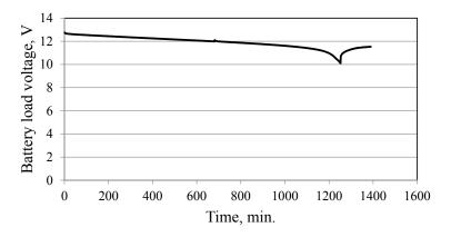
Figure 17. Battery discharge voltage behavior without the smart controller.
