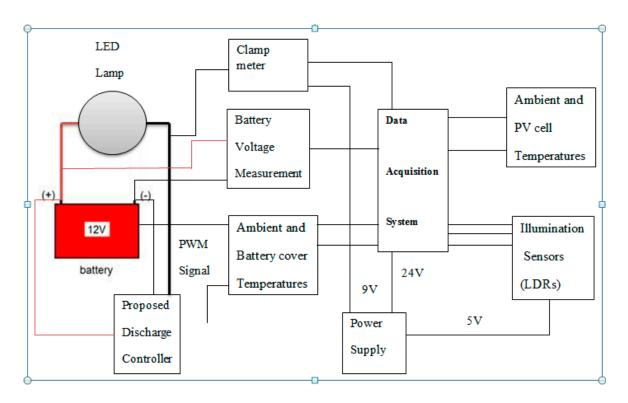
Figure 12. Schematic diagram of the experimental setup.
