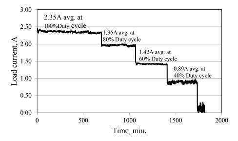
Figure 14. Variation of load (discharge) current during system operation with the smart controller.
