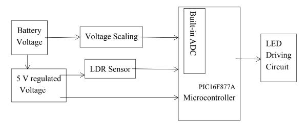
Figure 3. Block diagram of the proposed smart discharge control system.
