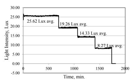
**Figure 16.** Variation of light intensity at the floor directly under the LED and 6 m away with using the smart controller.
