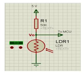
Figure 7. Schematic diagram of the LDR sensor.
