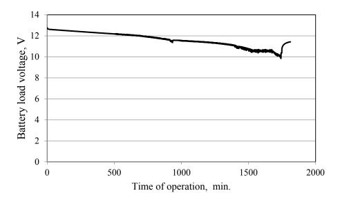
Figure 13. Variation of battery voltage during system operation with the smart controller.
