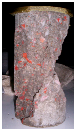
Figure 5. Failure surface of recycle brick concrete.
