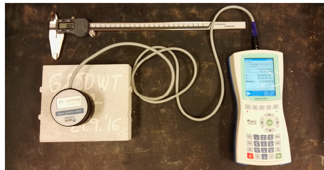
Figure 2. Thermal conductivity measurement of cement composites based on recycled waste paper.
