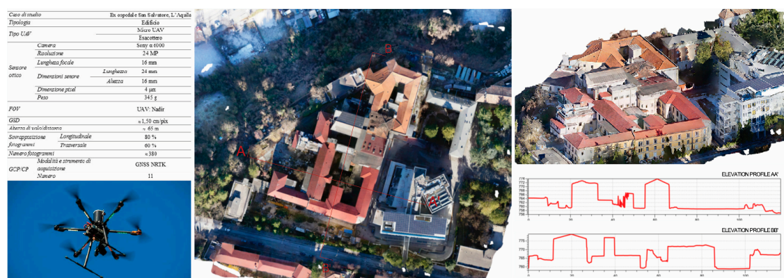
Figure 6. Unmanned aerial vehicle (UAV) photogrammetry. From left to right: features and views of the used vehicle; orthophotograph of roofing, three-dimensional reconstruction and elevation profiles obtained from the UAV campaign.
