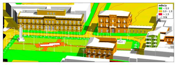
**Figure 4.** Pompei, Bartolo Longo Square. CIM axonometric view, towards south side, categorized with Yearly Equivalent Dose proceeding from flooring building materials.
