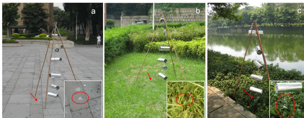
Figure 2. Details of the measurements for air temperature/humidity profiles, surface temperature, and grass leaf temperature: (a) granite slab pavement; (b) shrub + grass; and (c) beneath trees.
