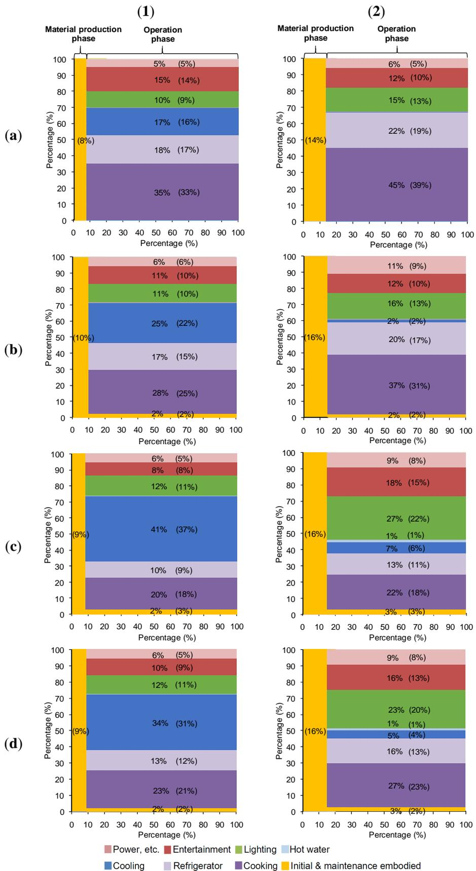
**Figure 11.** Contribution to CO<sub>2</sub> emissions by end-use in the whole building's lifespan for respective house categories in (1) Jakarta and (2) Bandung for Scenario 1: (a) simple house; (b) medium house; (c) luxurious house; and (d) whole sample. Note: The percentages in the parentheses show the contribution to CO<sub>2</sub> emissions by end-use in the whole building's lifespan.
