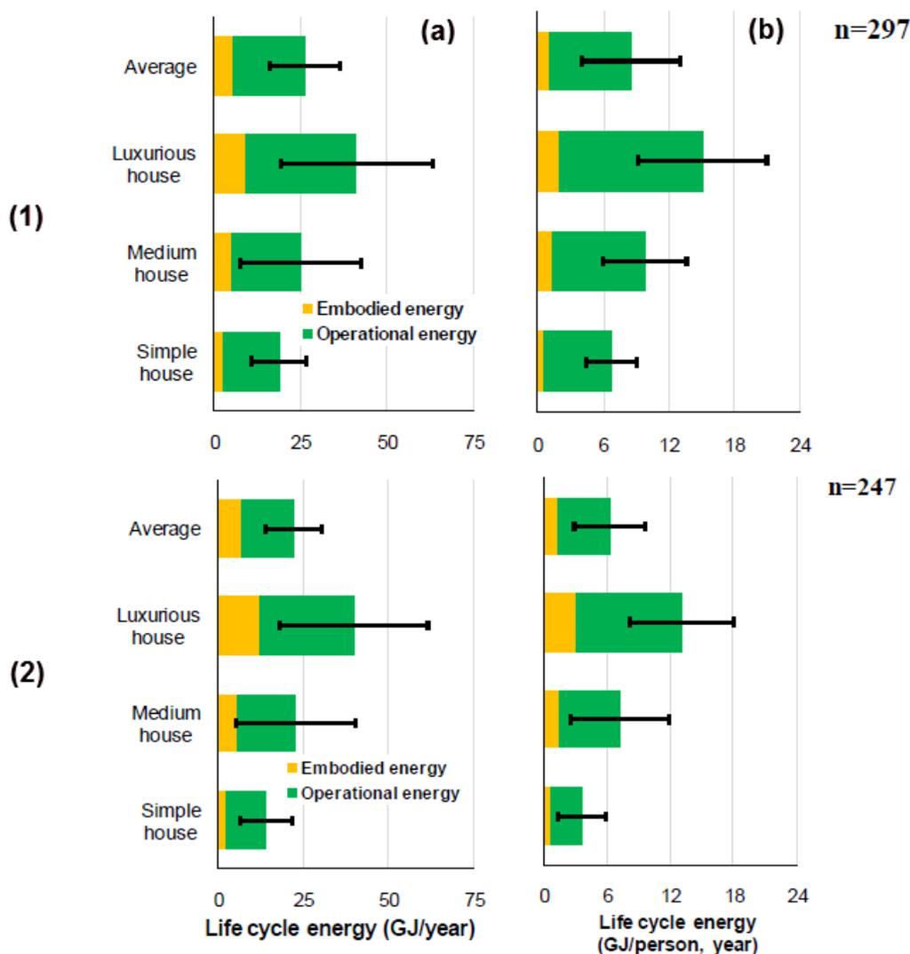
**Figure 9.** Average annual life cycle energy for respective house categories in (1) Jakarta and (2) Bandung for Scenario 1. (a) Total life cycle energy and (b) unit life cycle energy (per person). Note: The error bars indicate the mean values  $\pm$  standard deviation.
