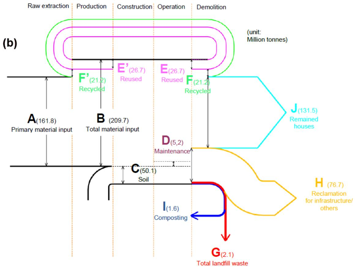
**Figure 4.** Flow of building materials for individual houses in Jakarta by 2020 (all houses): (a) Scenario 1 and (b) Scenario 2.
