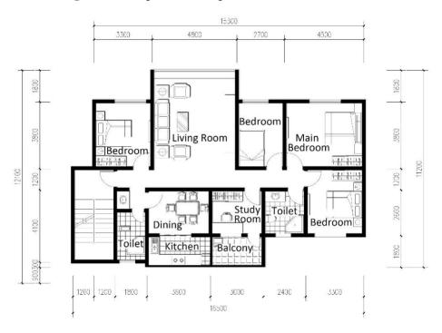
Figure 4. The plan of the apartment after modification.
