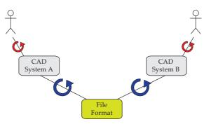
Some file formats contain animation data, some describe building components, others are used for interactive web applications, and so forth. Because a different part of the AEC domain is described in each of these file formats, each file format tends to use a partly unique structure with an equally unique
