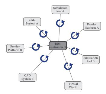
Although this approach appears to eliminate some interface points, several such points persist in this approach (Figure 6). These interface points are, however, seldom included in overviews of this BIM
