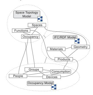
The second partial model, that should be closely linked to the first partial model, represents the building using the terms available in the IFC ontology, including geometric properties of the building and, to some extent, product information. It would presumably be a good test for the change propagation and change discovery features of the system to see to what extent changes in the IFC/RDF model of the building can be propagated into the space topology model (Figure 14).
