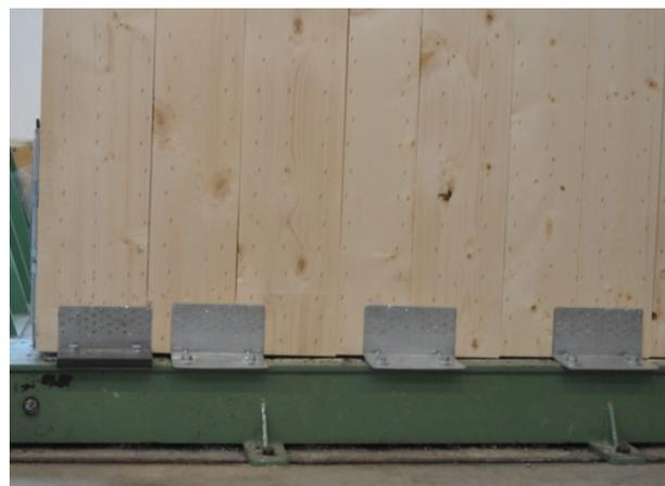
**Figure 13.** Wall C: Shear deformation between vertical boards at end of testing: (a) Front face; (b) Rear face.
