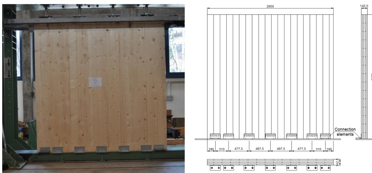
Wall B was fixed to the foundation with seven angular steel elements (Titan TCN 240, Rothoblaas, Cortaccia (TN), Italy) positioned as shown in Figure 3. Two configurations were prepared: Titan Type A has a thick steel plate between the bolt head and the angle bracket, placed at the edge of the panel as
