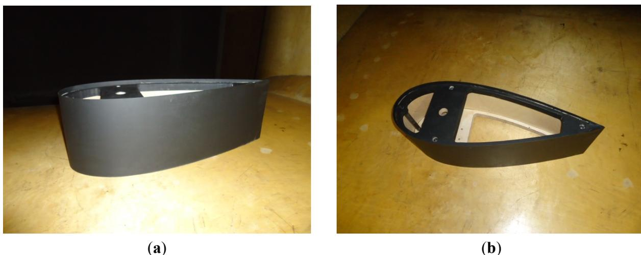
Similarly, the 1:10 scale model of the typical construction load, the “Brick”, was built with the same technique, having a chord length of 600 mm, maximum width of 210 mm and height of 200 mm, giving a reference area of  $0.043 \text{ m}^2$ .
