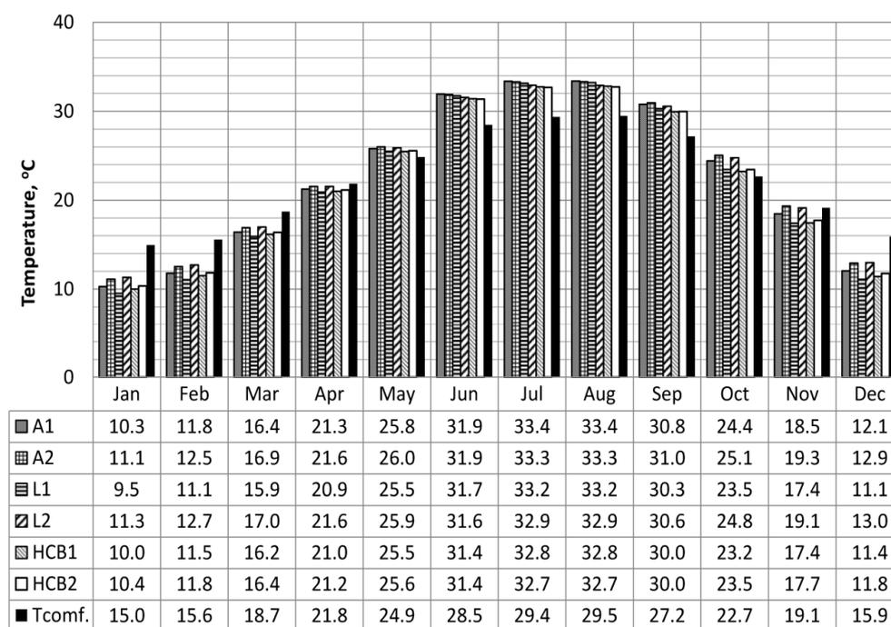
Annual performance of wall types is presented in Figure 8, which indicates the deviation of  $T_{in}$  from  $T_{comf.}$  in summer (positive) and winter (negative) for an entire year. The summary of dynamic thermal properties for the six wall types (Table 4) shows that walls HCB1, HCB2 and L1 have higher decrement factors resulting in greater indoor temperature swings with relatively short time lags and lower effective thermal mass.
