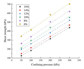
Figure 3. Shear strength of samples of soil with varying levels of moisture.
