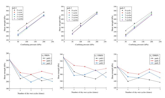
Figure 7. Peak shear strength of soil samples under different wet and dry cycle paths.
