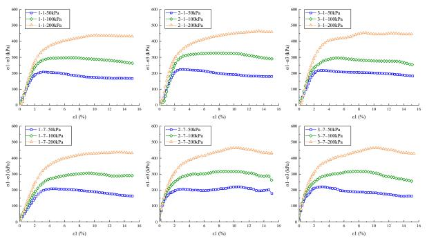
Figure 5. Soil sample stresses and strains under various conditions and the quantity of wet-dry cycles.
