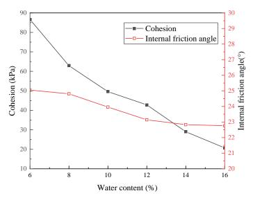
Figure 4. Impact of the amount of moisture on clayey sand's shear strength index.
