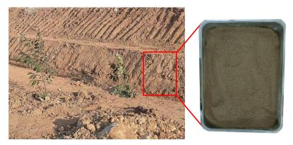
**Figure 1.** Untreated soil specimens and the expansion site of the Rongwu Expressway's Weihai–Yanhai section.
