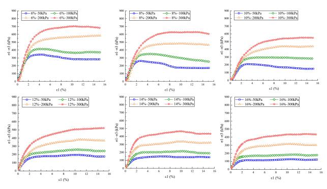
Figure 2. Curves of stress and strain for clayey sand with different moisture contents.
