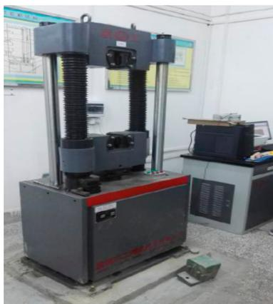
**Figure 3.** Material mechanics universal testing machine.
